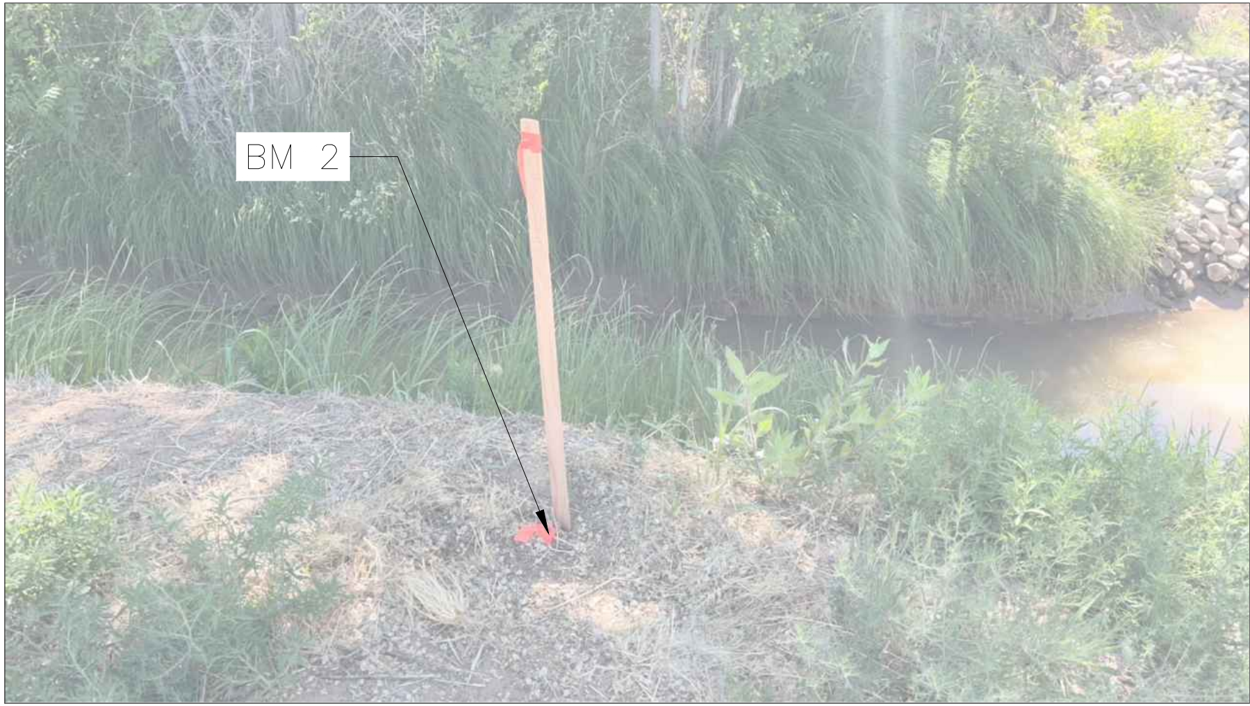
BENCHMARK 2 (BM2): DESCRIPTION: BM2 IS LOCATED NEAR THE WEST BANK OF CHICAL LATERAL AT STATION 311+50. THE BENCHMARK IS MARKED BY A REBAR WITH ORANGE FLAGGING AS SHOWN IN THE PHOTO ABOVE. NORTHING: 1395857.3639' EASTING: 1514634.7485' ELEVATION: 4875.08'
