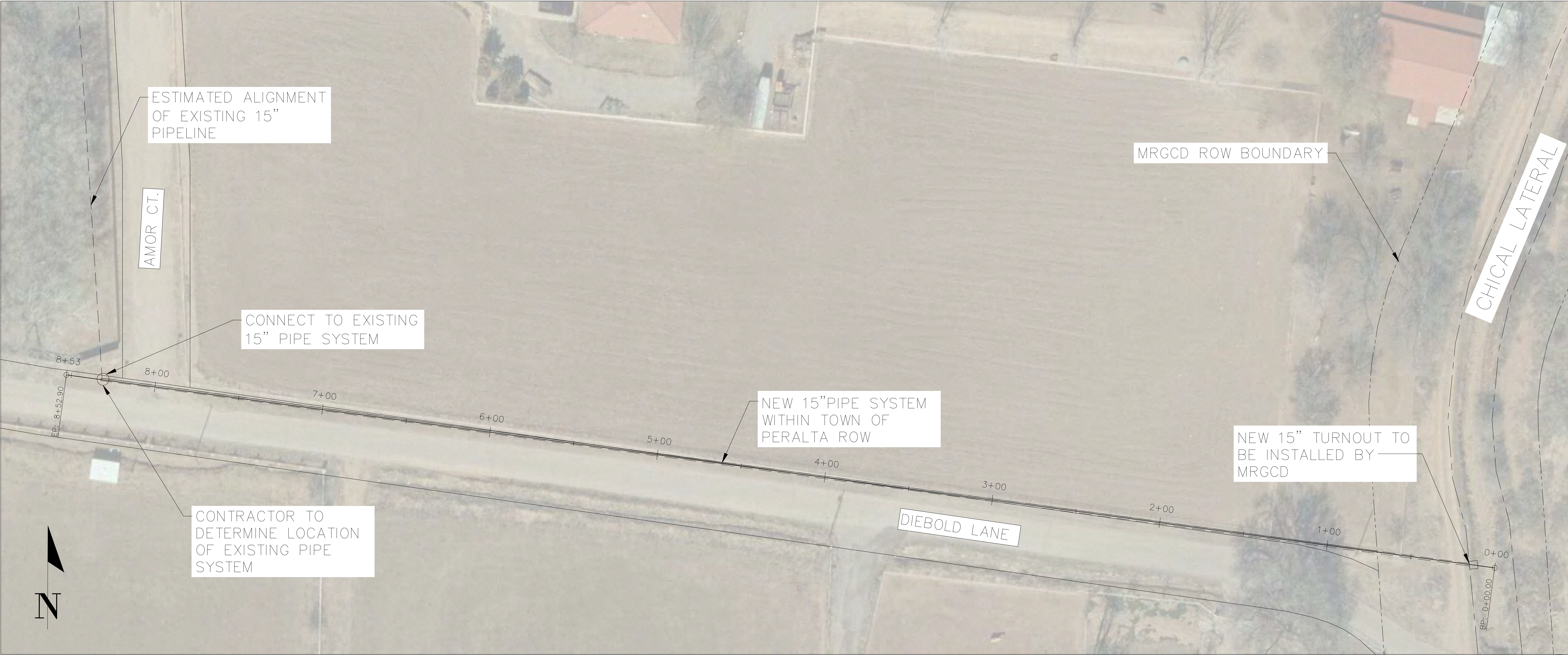
PIPELINE PLAN VIEW SCALE 1"= 30'
