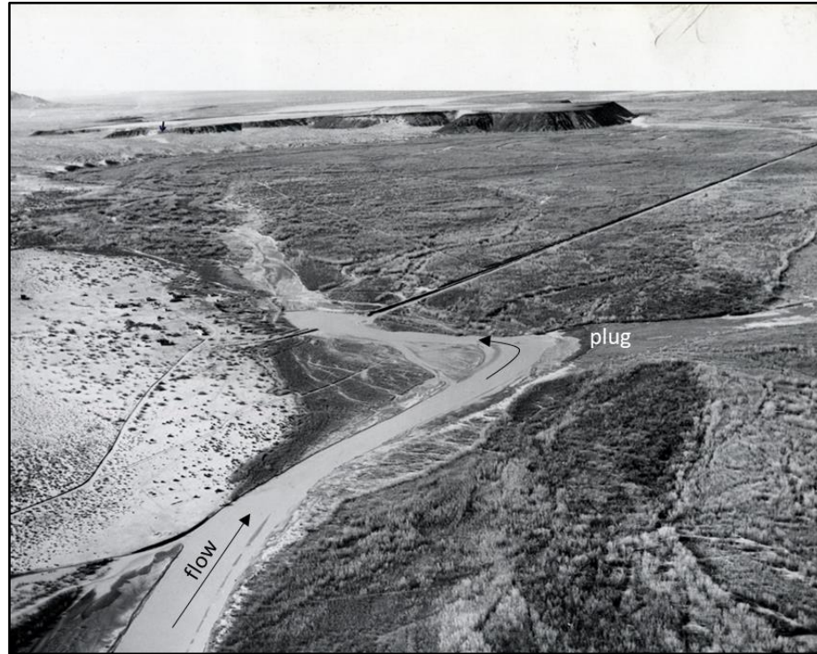
Aerial photo from 1952 showing the river altering course due to a sediment plug forming within the San Acacia Reach above the Tiffany Basin.
